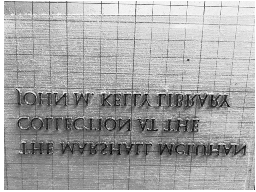
A photopolymer plate on a bedplate at the Kelly Library Print Studio. (Deborah Barnett photo)
